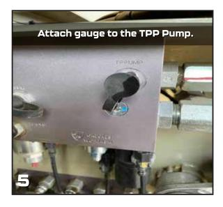
Break jam nut loose with a 3/4 wrench and insert a 1/4 hex key on the RV1 Pump Relief - Turn on PTO Pump. Now turn the hex key clockwise. At the same time, press and hold the minus symbol on the machine angle option until the gauge reads 2200-2250 PSI. Once your gauge reads the right PSI, turn off PTO Pump and lock the jam nut on RV1 Pump Relief. NOTE: Best to have two people for this step. This step is primarily done when completing the initial set up on the machine.
