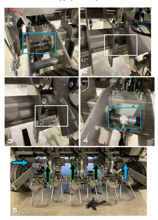
**NOTE:** The spacing from center wheel to wheel is set to 80", unless otherwise shifted before. It is recommend that you mark off the spacing of the brackets (with a paint pen) before you begin shifting.
