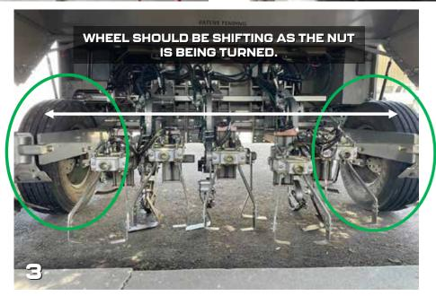
**STEP 4:** Once the wheels are properly spaced, tighten all of the nuts and bolts on the gauge wheel bracket that were loosened.
