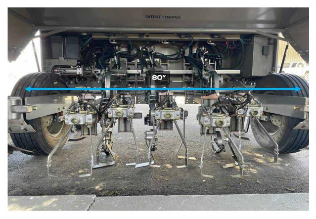
Shift each wheel in the same increments. For example: If you are setting your wheel spacing to 84" from 80", move each wheel out 2". If you are setting your wheel spacing to 76" from 80", bring each wheel in 2".
