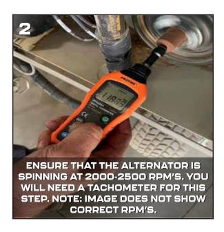
Once this is done, the "Volts" readout on the Control screen should read no less than 13.8v. If volts are less than 13.8v, the machine will not function properly.
