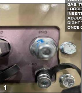
TURN OFF PTO. ATTACH TEST GAUGE TO GAS. TURN ON PTO. BREAK NUT ON PR8 LOOSE BY USING THE 9/16 WRENCH AND INSERT THE 5/32 HEX KEY INTO THE ADJUSTMENT STEM. TURN LEFT OR RIGHT TO SET 750 PSI. TIGHTEN NUT ONCE COMPLETE.
