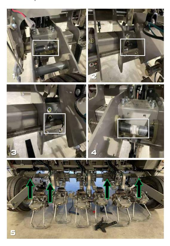
After completing the previous step, the following steps will require movement of the backbones. Base your measurements from the inside of the gauge wheel brackets, which are roughly 70" apart. When you begin to bring in backbone 2, you will want actuator 4 to sit at the corner of the 70" - at 35". Actuator 4 will be your center reference when spacing out the rest of the actuators.
