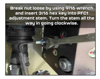
Break nut loose by using 9/16 wrench and insert 3/16 hex key on PR's 2-8 (Cultivator arm, back pressure, side shift) - turn stem counterclockwise all the way
