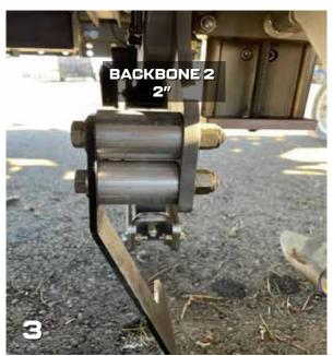
**STEP 9:** Once the backbones are centered, you can now begin to tighten all of the nuts that were loosened in the previous steps. Refer to the previous pages. Ensure that everything is tightened, otherwise brackets may shift and cause spacing confusion.
