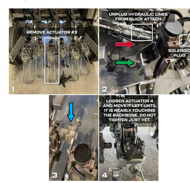
**STEP 2:** Backbone 1 will need to shift right. Backbones 2 & 3 will need to shift left. In order for them to shift, break loose the back plate on the 2" bar and the 4 bolts on the 4" bar - this will require crawling under the machine. You will need a 15/16" wrench and best to also have a 15/16" deep socket and ratchet.
