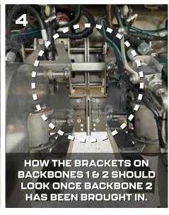
**STEP 5:** *NOTE: Having 2 people for this step is best.* Center actuators 5 & 6 on backbone 3 to what the line spacing of the field is. Once that is done, move backbone 3 to the left (follow the same steps as the previous slides) until you reach the desired line spacing between actuators 4, 5 & 6.
