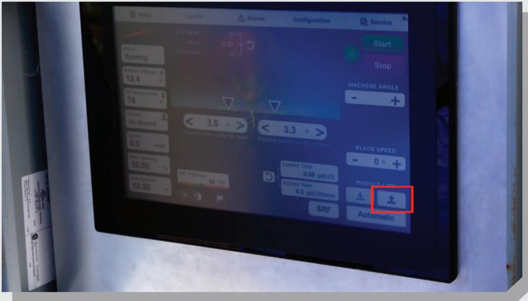
**STEP 09:** Verify SRF pump pressure equals 60-70 PSI. Check the digital reading in the bottom left of the control screen, or check with a physical gauge to ensure the pressure is between 60-70 PSI.
