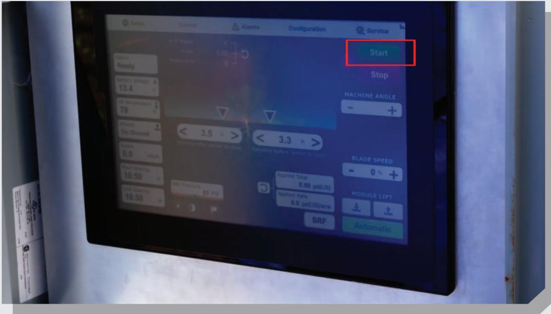
**STEP 08:** Press UP arrow to prepare Backbones. Backbones UP, Backbones valves LOCKED.
