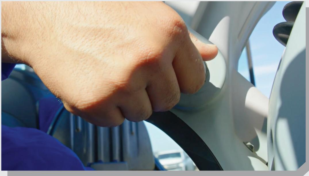
**STEP 04:** Engage tractor hydraulic valve -
